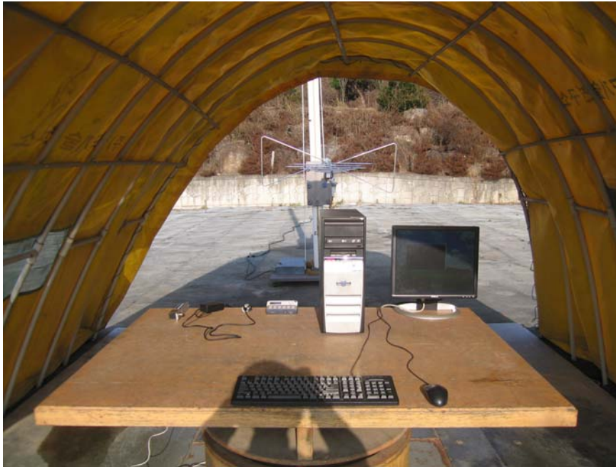
Photograph 2 : Setup for radiated Emissions (above 30 MHz)
