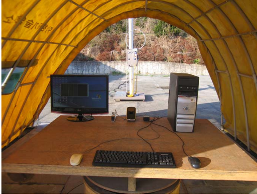
Photograph 2 : Setup for radiated Emissions below 30MHz
