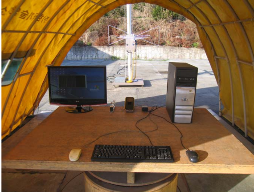
Photograph 1 : Setup for radiated Emissions 30MHz to 1GHz
