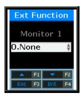
Set when connecting an external contact to DM0. (When using a motor lock, set to 1 or 2.) Default Setting: '0.None'
