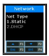
Select [1] if Static IP is assigned, and select [2] to set IP using DHCP.
