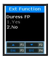
Set whether to use the duress fingerprint alarm. Default Setting: '2.No'
