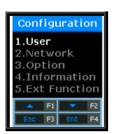
Select the menu you want to change using  $[\uparrow](F1)$  and  $[\downarrow](F2)$  buttons, and press [ENT] (F4) button to go to the submenu.
