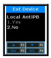
Default Setting: '2.No' When setting to '1.Yes', the Anti-Passback in the terminal is checked.
