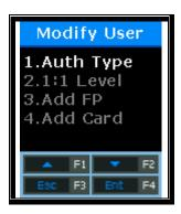
Select [1] to change the authentication method; [2] to modify the authentication level; [3] to add the fingerprint to the relevant ID; and [4] to add the card.
