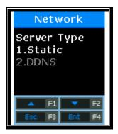
Select [1] if Static IP is assigned, and select [2] to set IP using DDNS.
