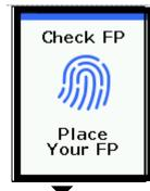
Place your finger on the fingerprint sensor, and the white light is on the fingerprint input window. Keep your finger until the white light is off with a beep sound.
