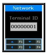
This ID is a unique ID used to allow the server to identify the terminal. The default is '00000001'. Default Setting: "00000001"
