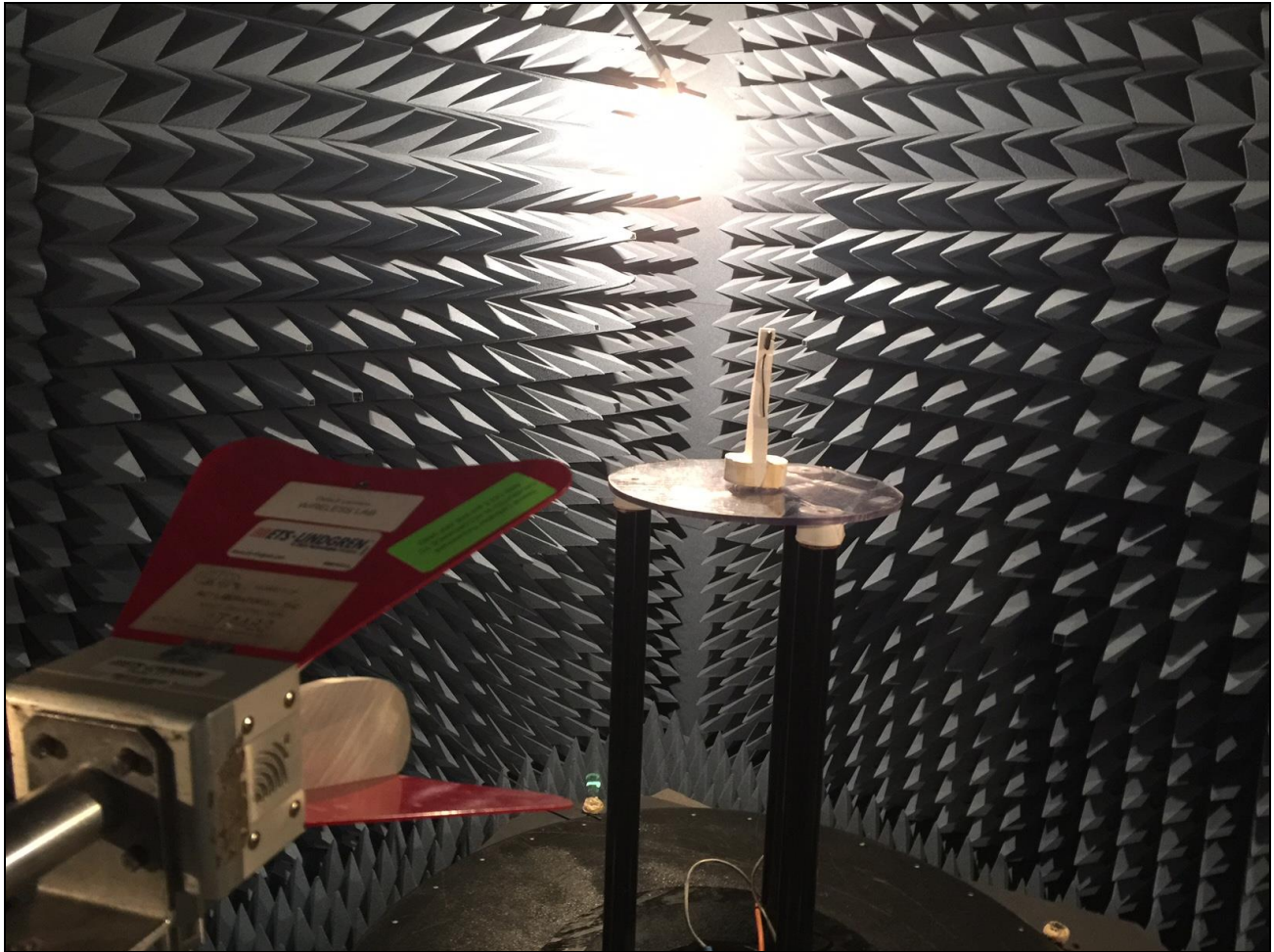
Photograph 2. Radiated Emissions, Test Setup
