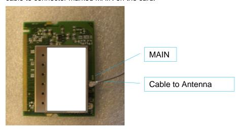
2.2 Align the notched end of the card with the socket. Insert the card into the socket.
