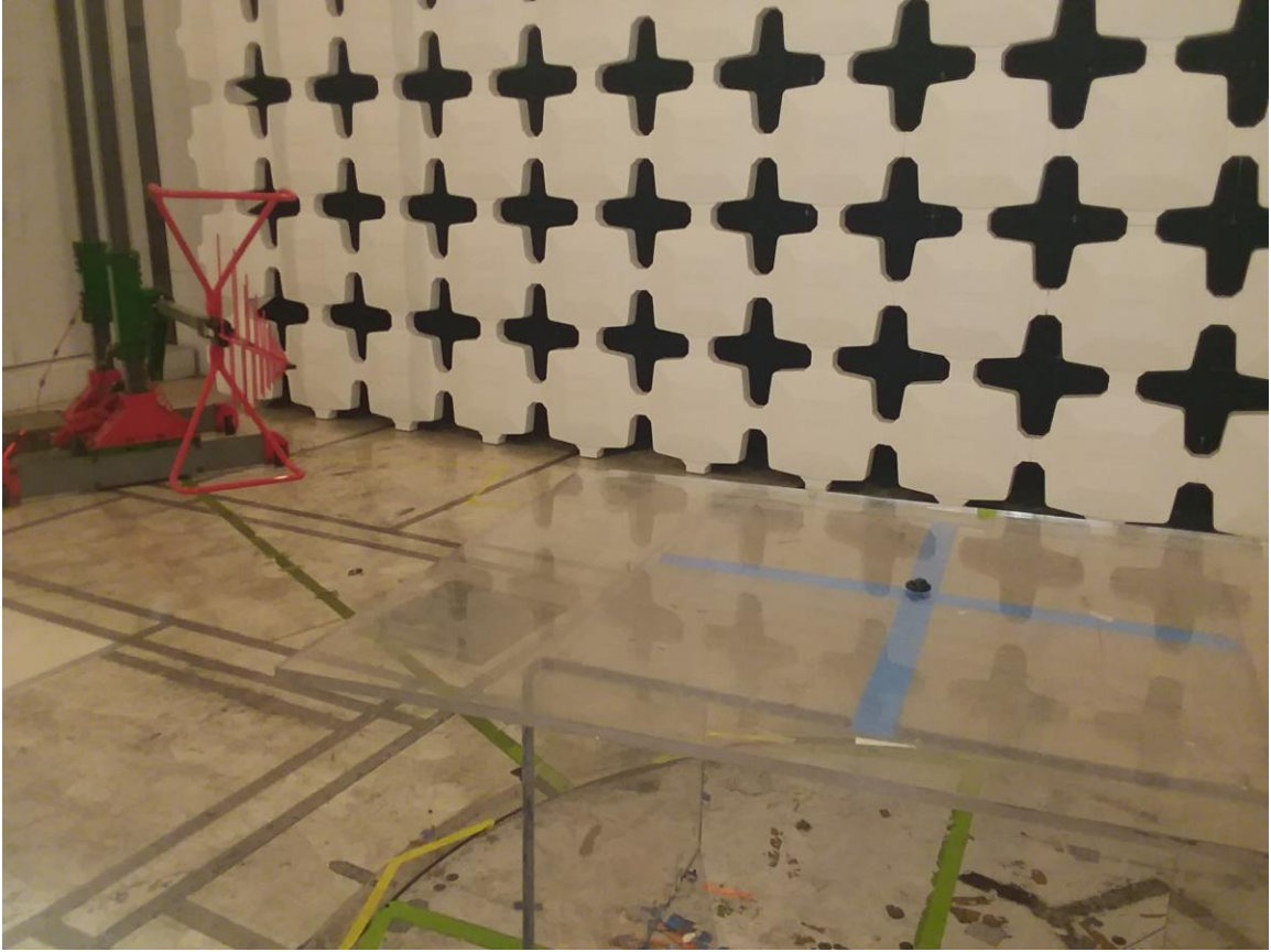
Photograph 2. Radiated Emissions, Test Setup
