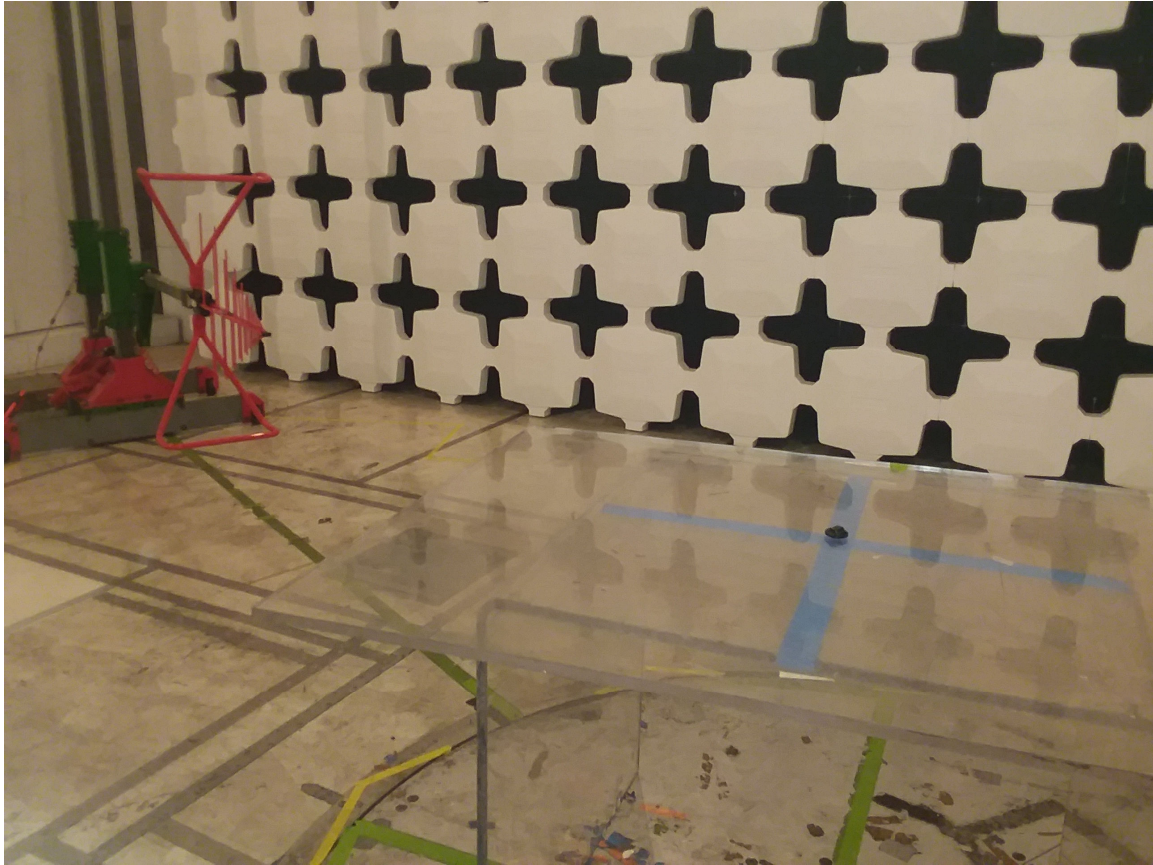
Photograph 2. Radiated Emissions, Test Setup
