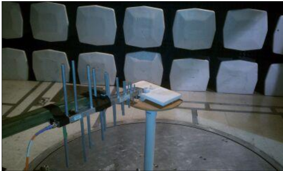
Photograph 2. 15.250(d)(1) Radiated Emissions, Test Setup, 960 MHz – 1 GHz
