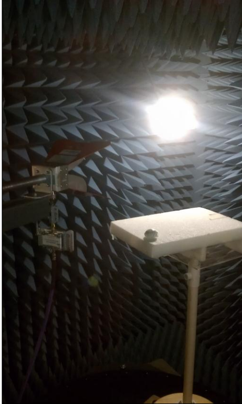
Photograph 3. 15.250(d)(1) Radiated Emissions, Test Setup, Above 1 GHz
