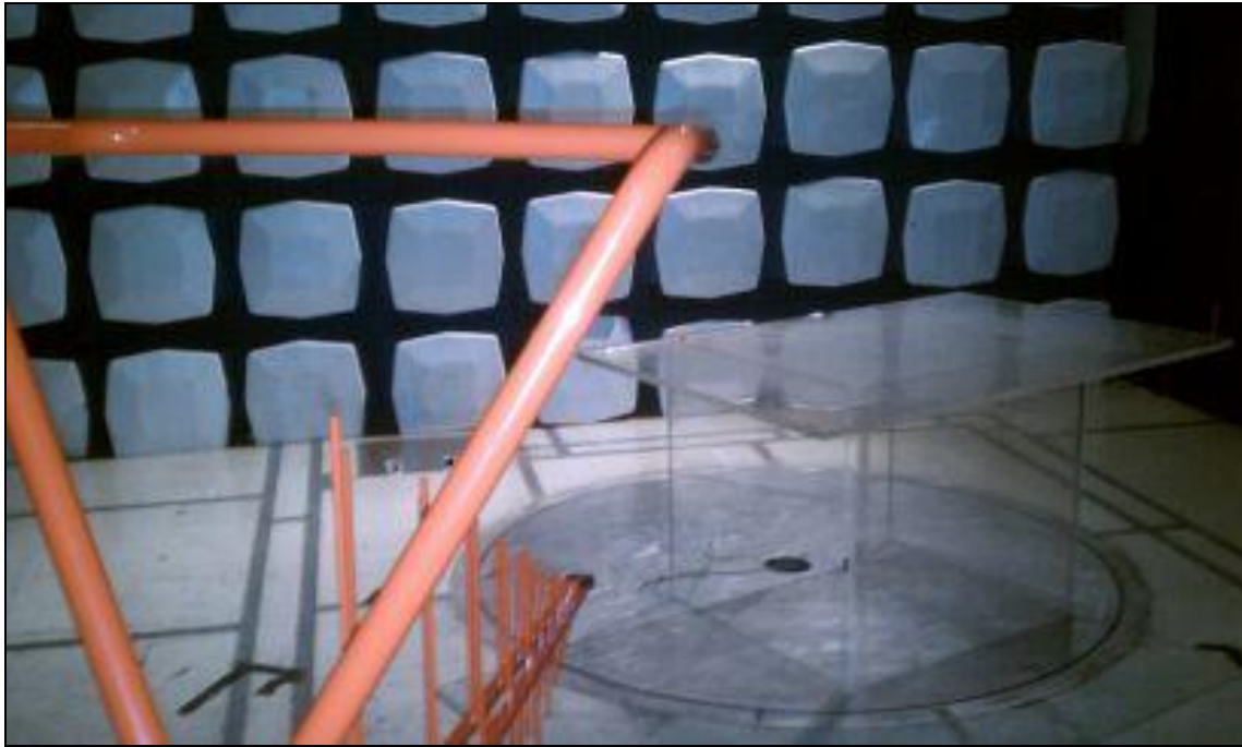
Photograph 6. Radiated Emissions, Test Setup, Below 1 GHz
