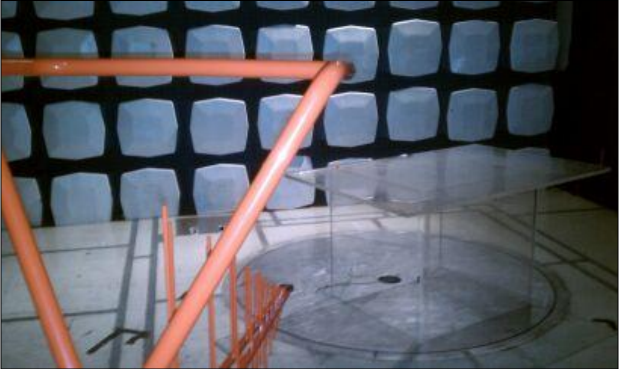
Photograph 2. Radiated Emissions, Test Setup
