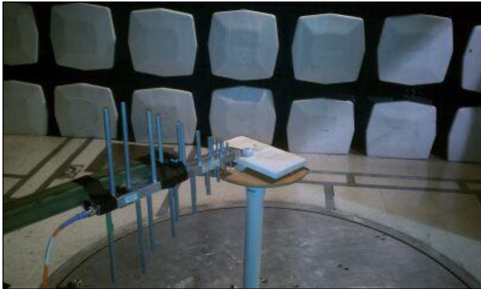
Photograph 3. 15.250(d)(1) Radiated Emissions, Test Setup, 960 MHz – 1 GHz
