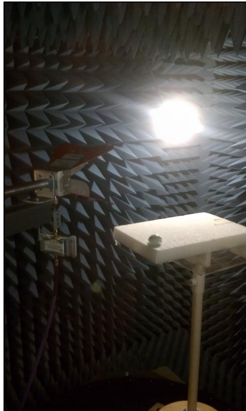
Photograph 4. 15.250(d)(1) Radiated Emissions, Test Setup, Above 1 GHz
