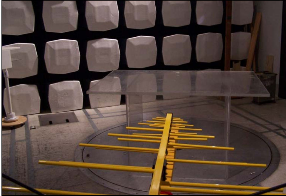
Photograph 1. RE Test Setup
