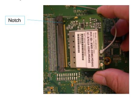
2.3 Push the card down until it snaps into the two retention clips.
