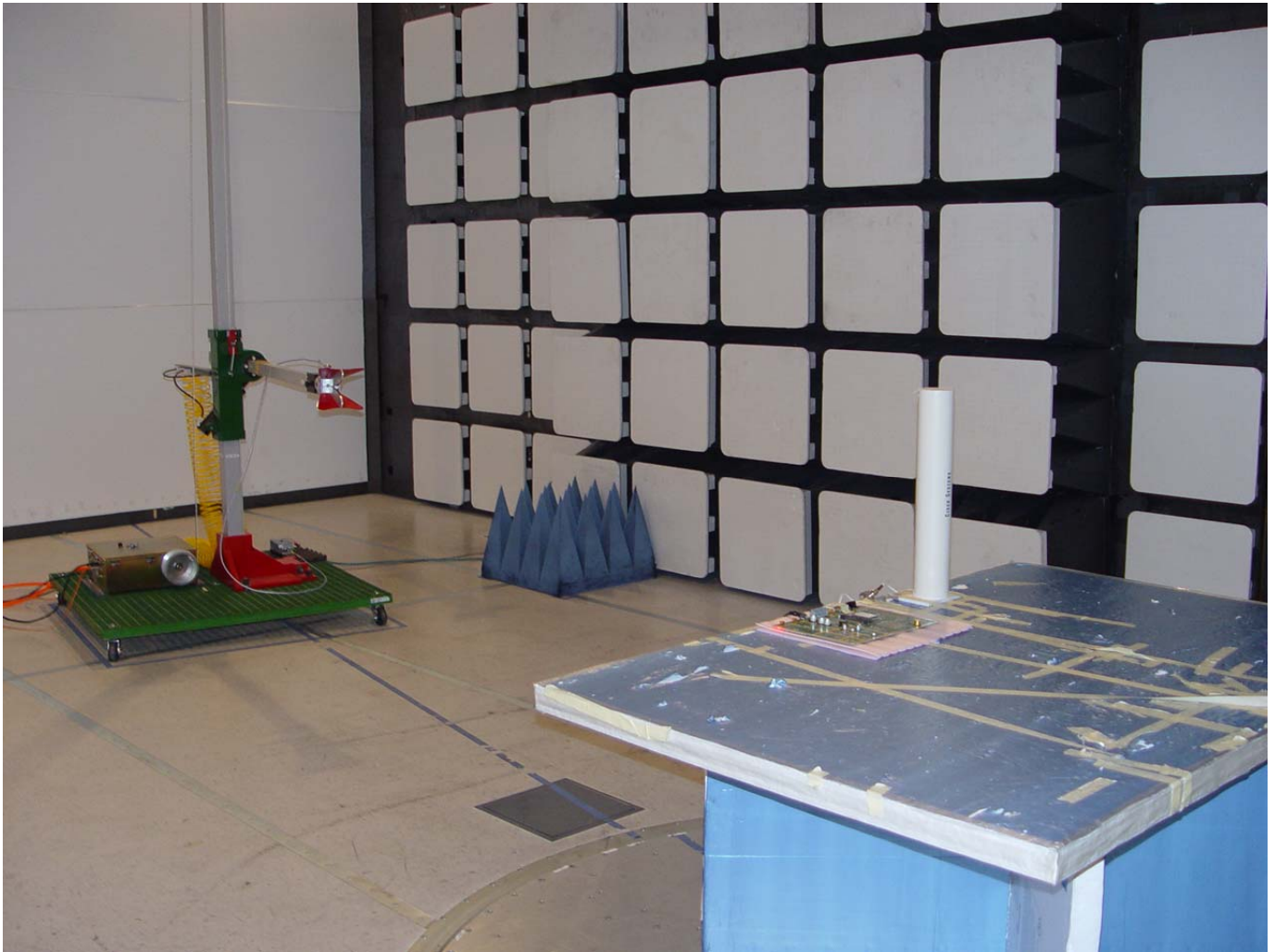
WiFi Module WLM54AG with yagi antenna AIR-ANT1949 (gain 13.5 dBi)
