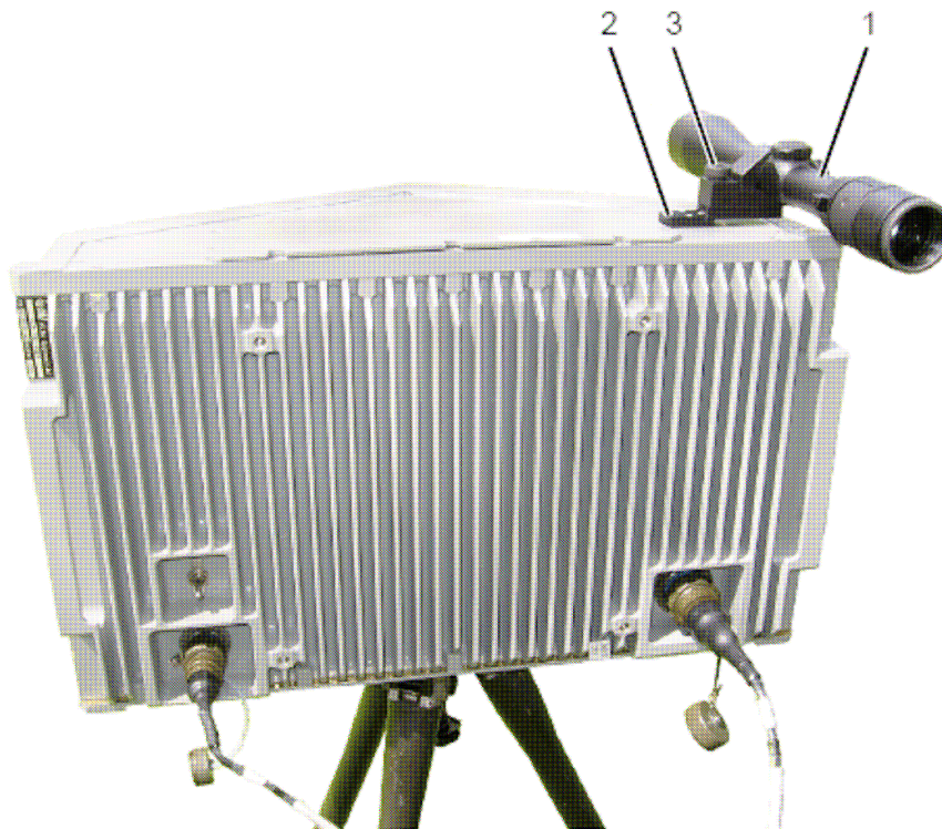
Figure 2-4. Aligning ELM-2127 Sensor Azimuth
