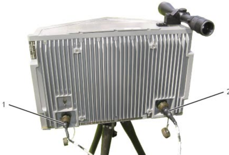
Figure 2-5. Connecting ELM-2127 Sensor to Tactical Center and Power
