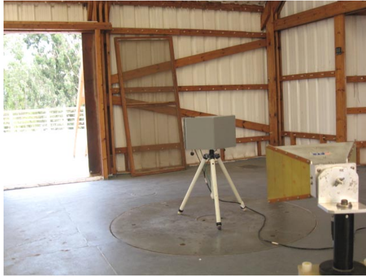
Photograph No.7 Radiated emissions measurement setup at the OATS above 1000 MHz
