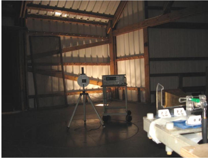
Photograph No.9 Setup for substitution ERP measurements of spurious
