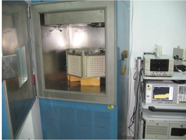
Photograph No.10 Frequency stability measurement setup
