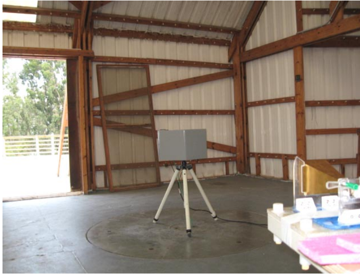
Photograph No.8 Radiated emissions measurement setup at the OATS above 1000 MHz
