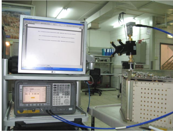
Photograph No.2 Conducted spurious emissions measurement setup
