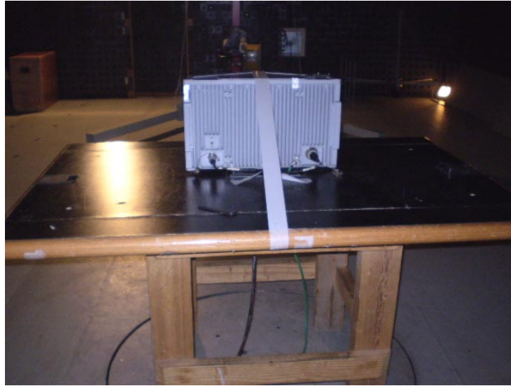
Photograph No.6 Spurious emissions measurement setup in the anechoic chamber, EUT close view
