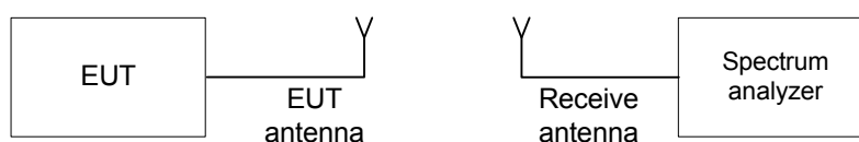
Figure 7.2.1 Occupied bandwidth test setup
