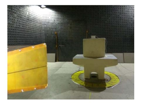
Photograph No.4 Radiated emissions measurement setup at the OATS in 18-40 GHz
