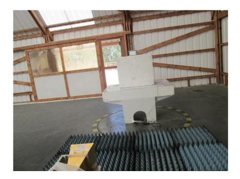
Photograph No.6 Occupied bandwidth measurements setup
