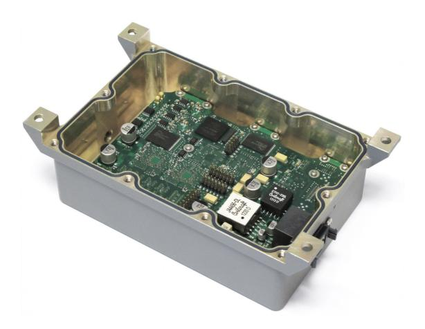
Photograph No.2 ELM 2114 radar removed from the case
