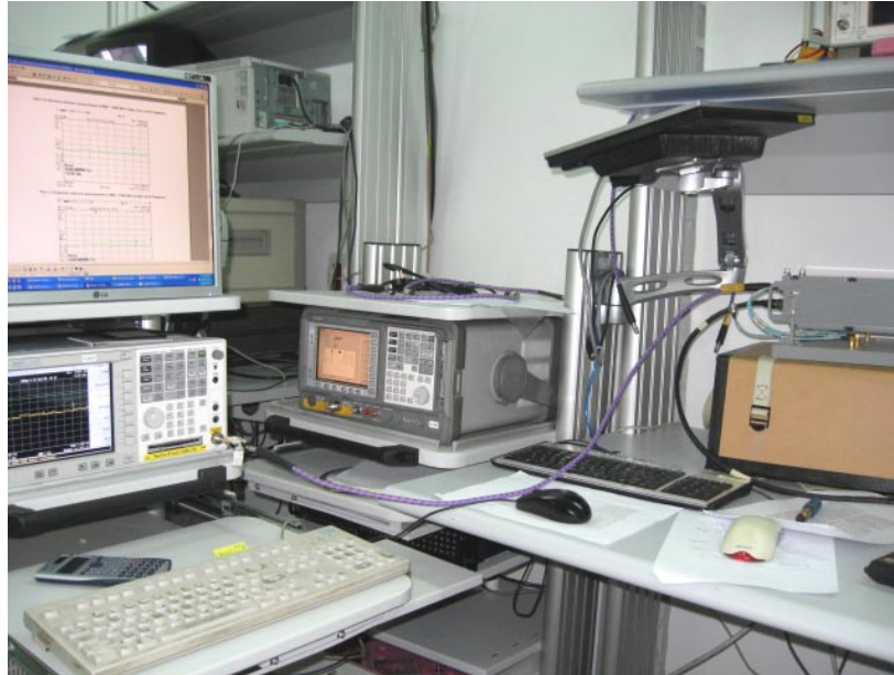
Photograph No.2 Occupied bandwidth, emission mask, conducted spurious emissions measurement setup
