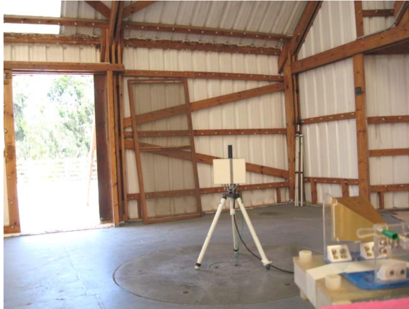
Photograph No.6 Radiated emissions measurement setup at the OATS above 1000 MHz
