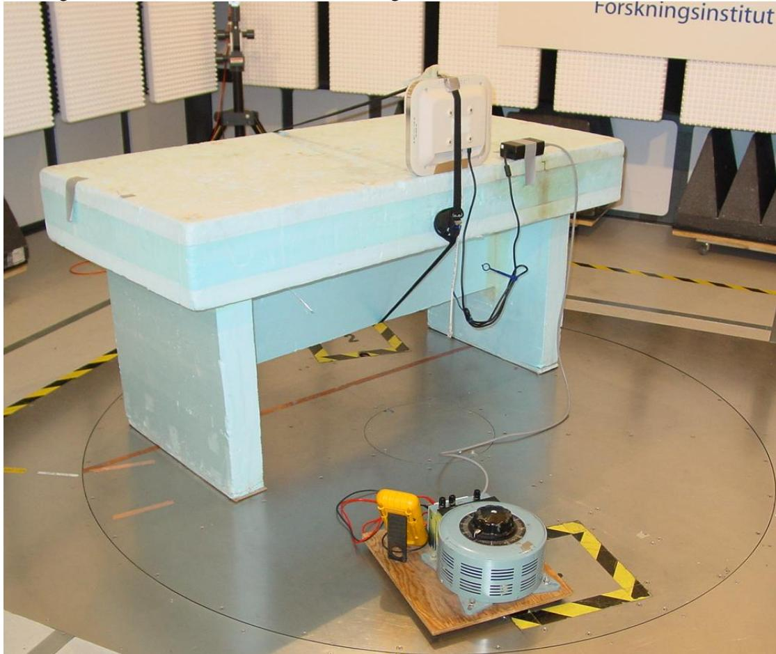
Note: The adjustable transformer and the multimeter were only used during the test of the Field strength of fundamental.
