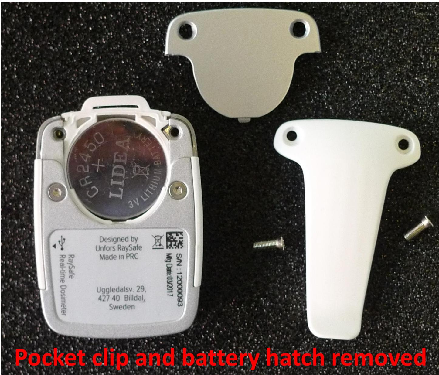
**Pocket clip and battery hatch removed**
