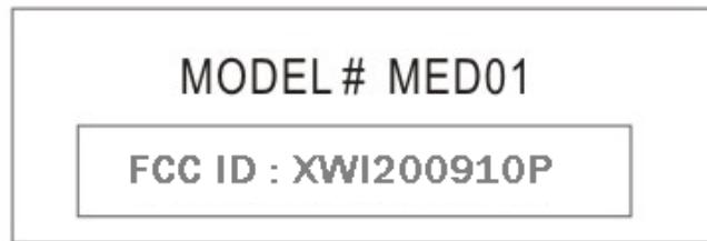
Specifications: Text is Black in color and justified. Labels are printed in indelible ink on permanent adhesive silk-screened onto the EUT or shall be affixed at a conspicuous location on the EUT.
