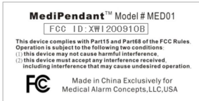
Specifications: Text is Black in color and justified. Labels are printed in indelible ink on permanent adhesive silk-screened onto the EUT or shall be affixed at a conspicuous location on the EUT.
