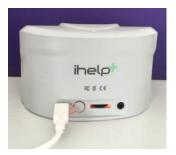
To release pairing, press the pairing button for 5 seconds until the pairing indicator light goes out.
