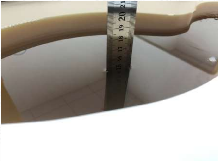
Picture 9.2-1 Liquid depth in the Flat Phantom for SAR measurements \leq 3 \text{ GHz}
