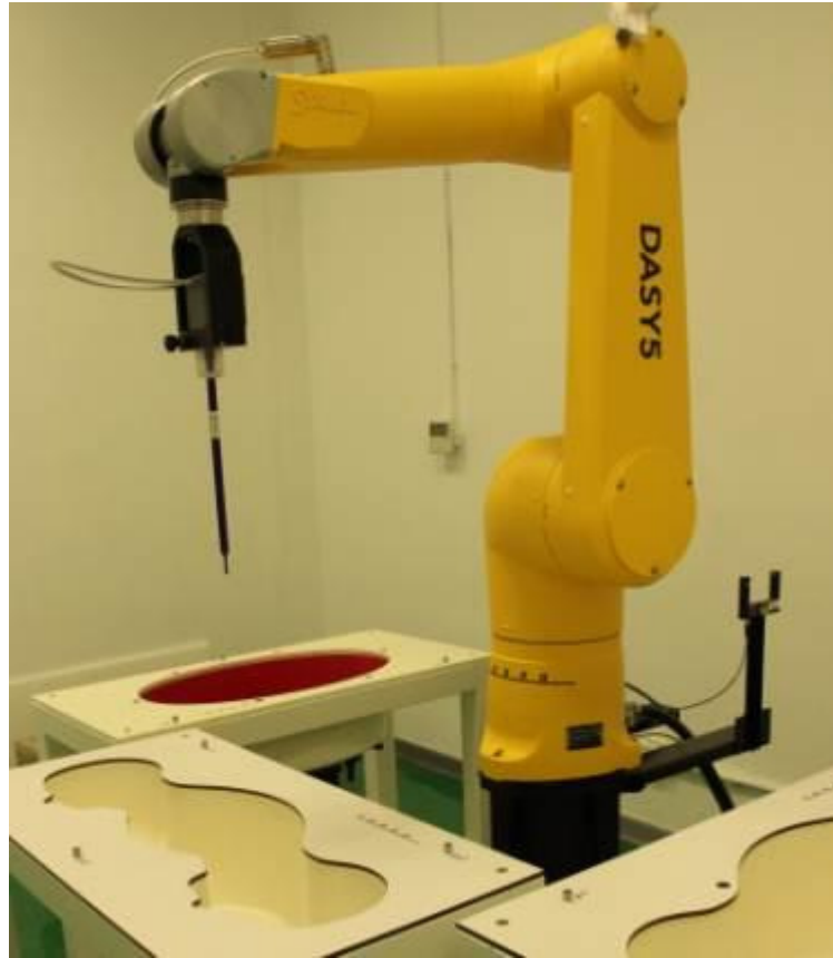
Picture D.6 DSY5 system Set-up
