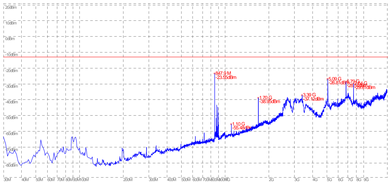
(Plot C.2: GSM 850MHz Channel = 251, Test Antenna Vertical)
