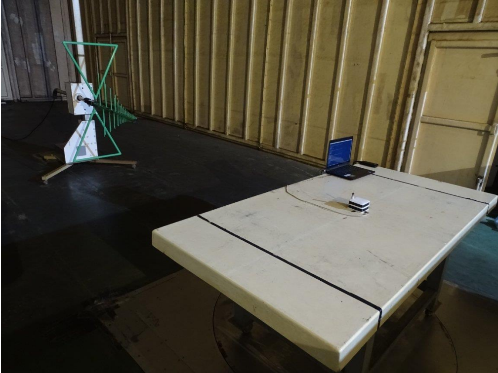
Front View of Radiated Test
