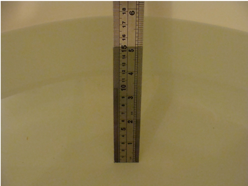
Depth of the liquid in the phantom
