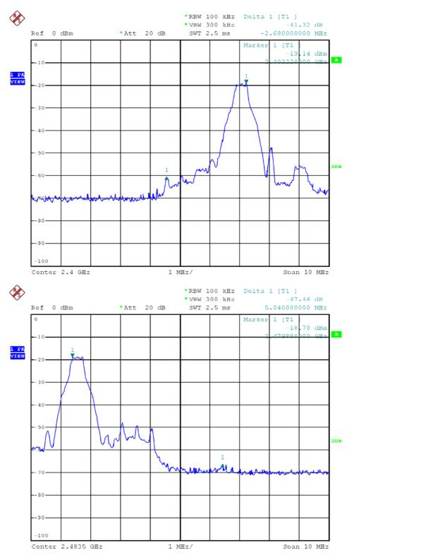
Bandwidth / Bandedge Plot – Pursuant to FCC Part 15 Section 15. 249 Requirement (Pass/Fail)
