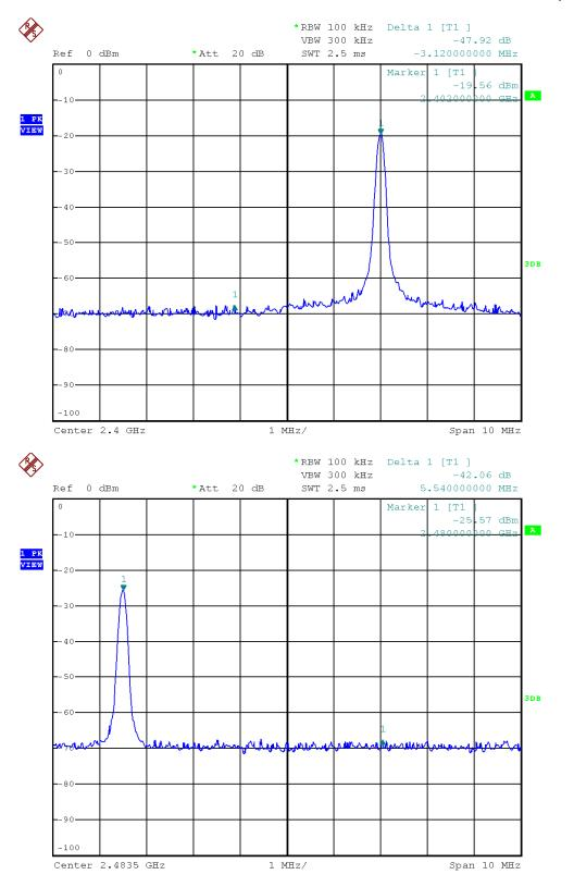
Bandwidth / Bandedge Plot - Pursuant to FCC Part 15 Section 15. 249 Requirement (Pass/Fail)
