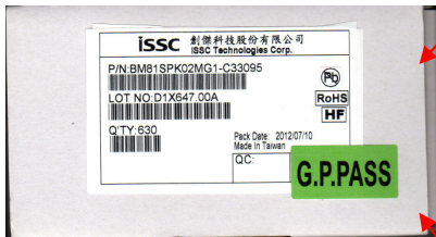
Bar Code Label P/N: SONY device name Lot No: Lot ID Q'ty: box or Carton Module's Q'ty
