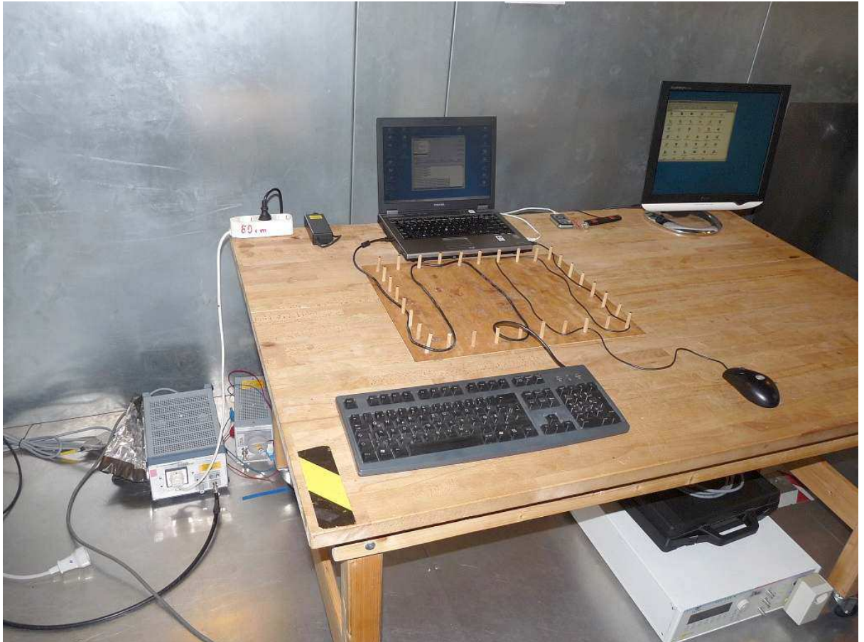
setup for conducted emissions test
