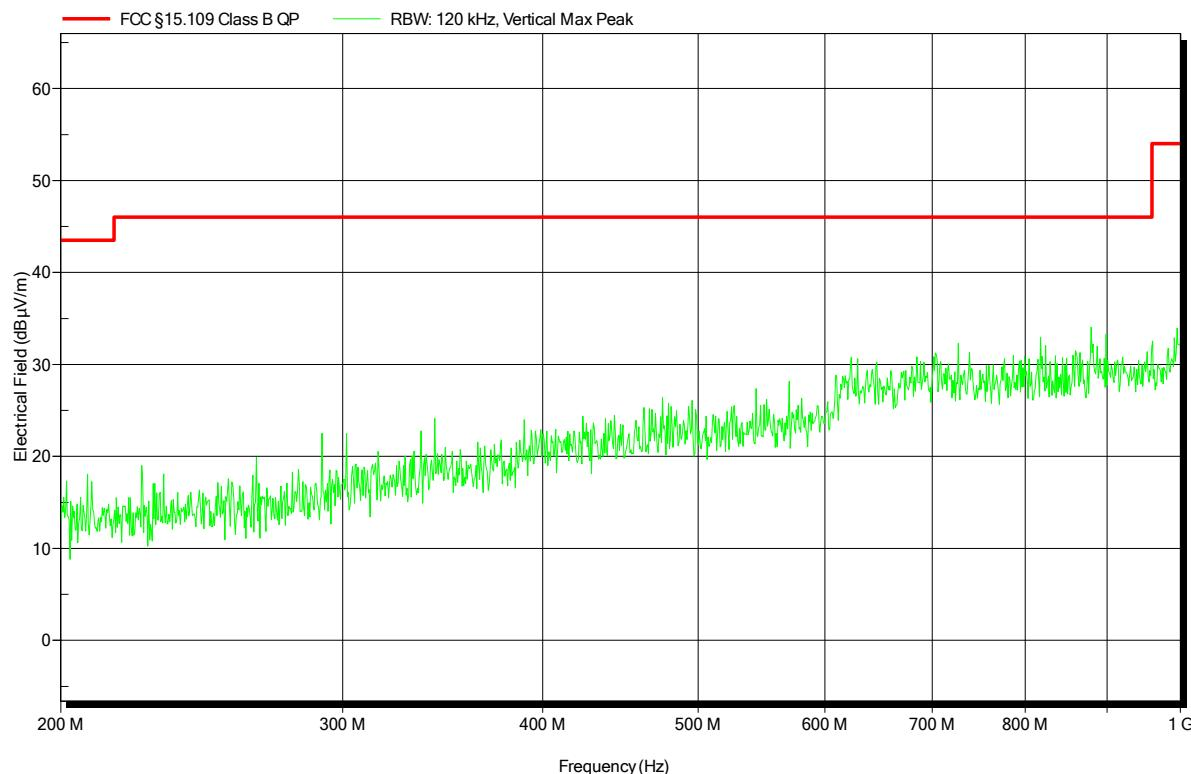
**Spurious emissions according to FCC part 15 Subpart C § 15.247, IC RSS-247, I1**
