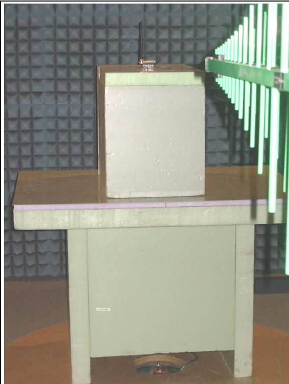
Figure 9: Measurement set-up for radiated measurement > 30 MHz and < 1 GHz acc. following sections of the report 1113-11-EE-11-PB001: 4.5.2 and 4.6.1
