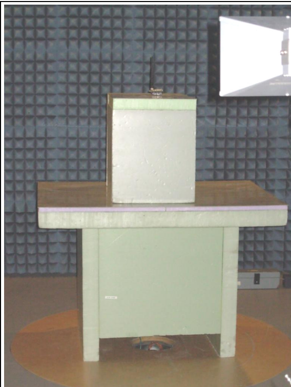
Figure 10: Measurement set-up for radiated measurement > 1 GHz acc. following sections of the report 1113-11-EE-11-PB001: 4.5.3; 4.5.4 and 4.6.2
