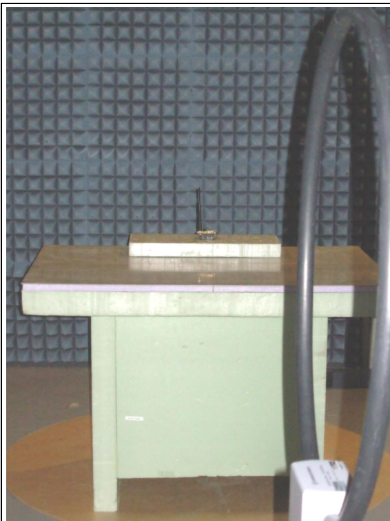
Figure 8: Measurement set-up for radiated measurement < 30 MHz acc. following sections of the report 1113-11-EE-11-PB001: 4.5.1
