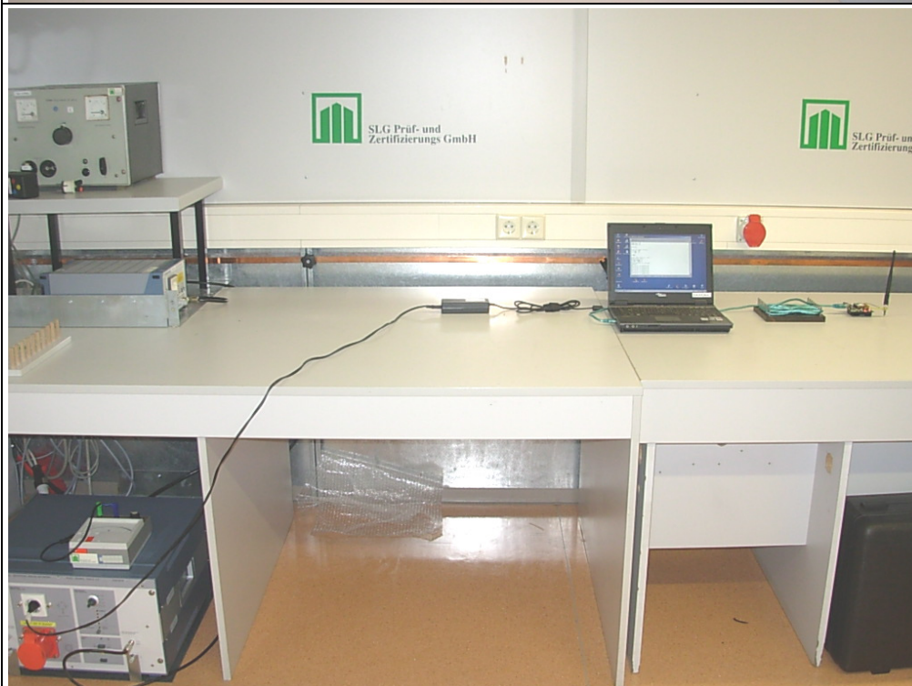
Figure 11: Measurement set-up for conducted measurement of disturbance voltage acc. following section of the report 1113-11-EE-11-PB001: 4.7 and 4.8
