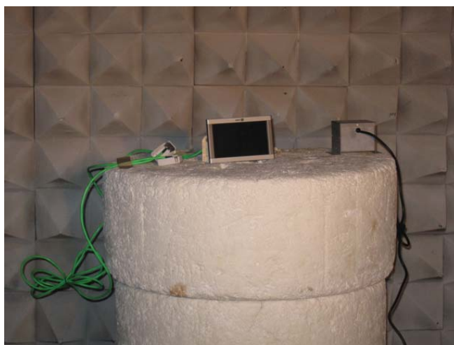
Figure 4: Radiated Emissions Test Setup Photograph(s).
