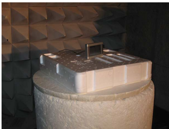
Figure 4: Radiated Emissions Test Setup Photograph(s).
