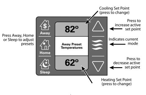
Use the **UP** and **DOWN** Arrows to adjust the Set Point to the desired temperature.
