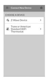
When prompted, prepare the device to be added to the Z-Wave network by following the device manufacturer's instructions to put device into add mode. You will have four minutes to complete this process.
