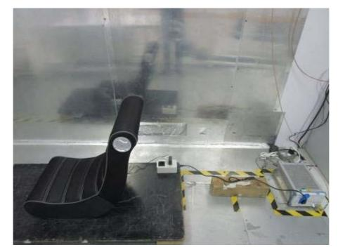
1.1 Conducted Emissions at AC Power Line (150kHz-30MHz) Test Setup
