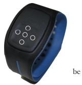
[Note: push the center button during time or date scroll to terminate scrolling text. When a menu heading is scrolling, pressing the center button will select that menu.]
