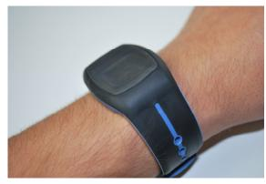
The ReadiBand is made of high-grade flexible plastic and is completely waterproof. The device may be worn in the shower, bath, or while swimming. It should be taken off when playing rough contact sports but otherwise should be worn at all times, including during light exercise. If the ReadiBand pod is damaged, the entire ReadiBand should be replaced immediately.
