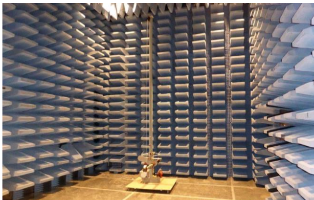
Chamber 2- 3m Semi-Anechoic Chamber (SAC) in Burnaby, BC
