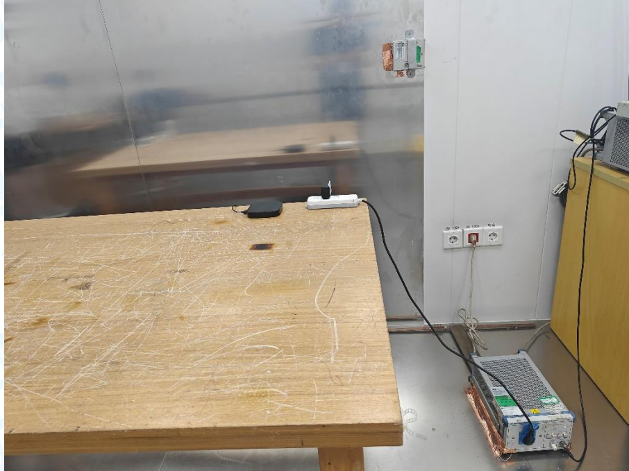
Photo of Setup for Radiated Emission (30MHz~1GHz)
