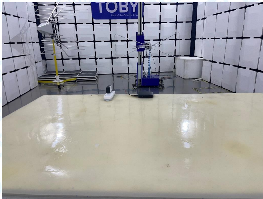
Photo of Setup for Radiated Emission (30MHz~1GHz)
