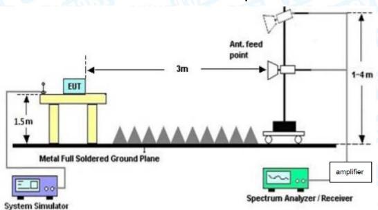
**Above 1GHz Test Setup**
