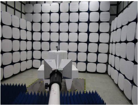
1.2 Radiated Spurious Emissions Test Setup
