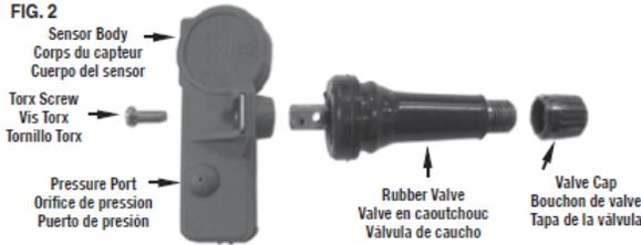
**For professional installation only:** Read and review all instructions, illustrations, and warnings before replacing existing sensor with new QWIK-SENSOR<sup>TM</sup>. Follow manufacturer recommended service and replacement procedures before installing. Improper installation may cause the Tire Pressure Monitoring System (TPMS) to malfunction.
