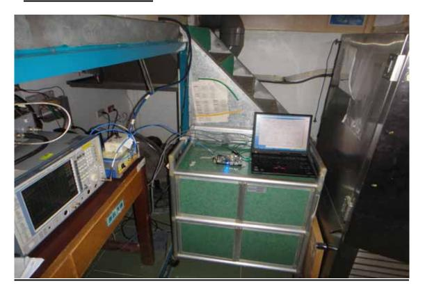
**POWERLINE CONDUCTED EMISSIONS MEASUREMENT SETUP**
