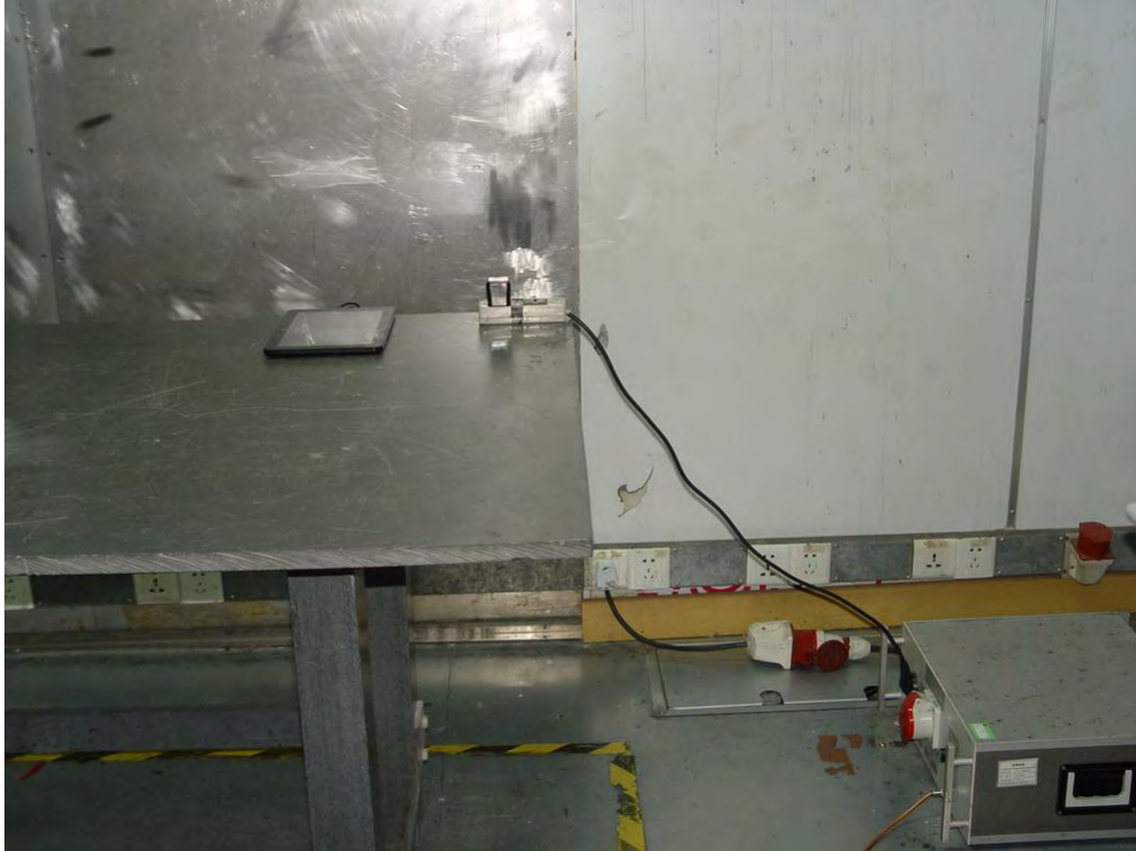
Photograph 2: Set-up for Spurious Emissions for below 30MHz
