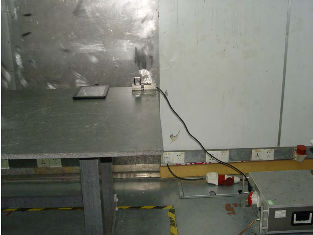
Photograph 2: Set-up for Spurious Emissions for below 30MHz
