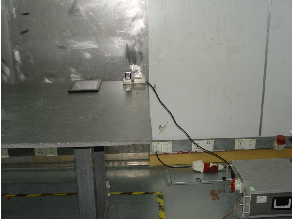
Photograph 2: Set-up for Spurious Emissions for below 30MHz
