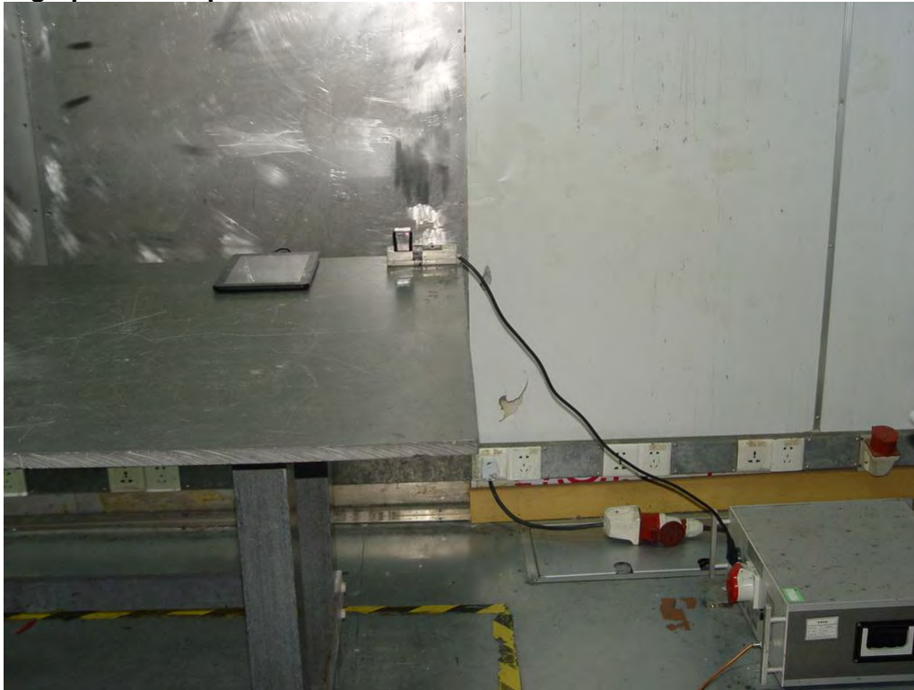
Photograph 2: Set-up for Spurious Emissions for below 30MHz
